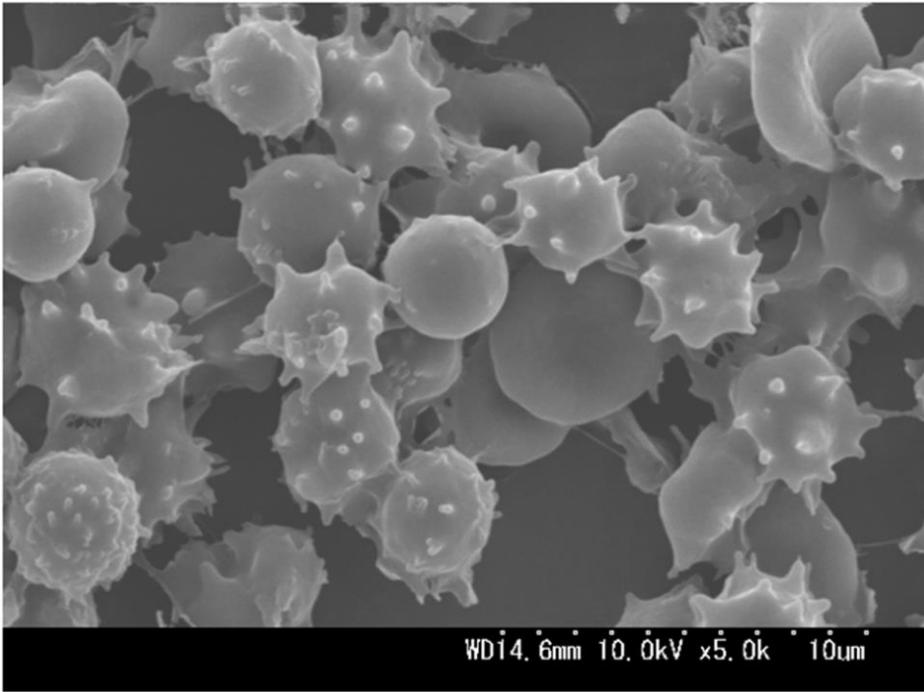
Figure 4 Echinocytes on the membrane oxygenator surface
