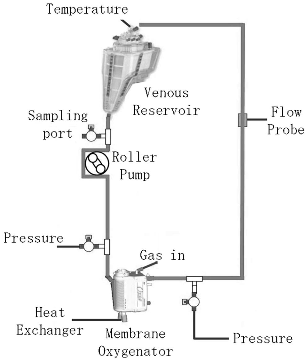
Figure 1 Experimental recirculation circuit
