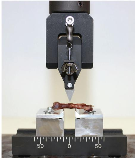
FIGURE 4: Three-point bending test.
